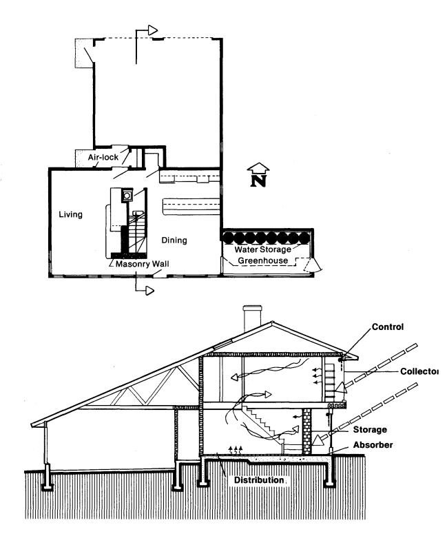
there is a first-floor greenhouse-adjacent to the dining room-with 120 square feet of south wall glazing. The greenhouse has 16 water-filled 55gallon drums inside its bermprotected north wall. All of these systems contribute to heating and cooling the house.
